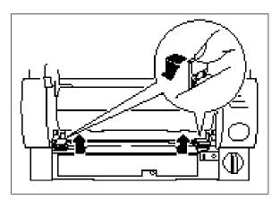
(4) Push the yellow colored tab of side cutter unit to release the lock as illustrated.
